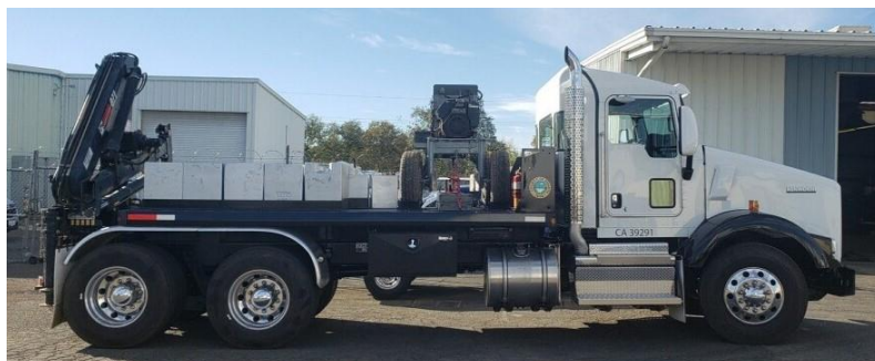
Shasta County Dept of Weights and Measures new weight truck. The individual weights seen on the bed of the truck are each certified to weigh 1,000 lbs.
