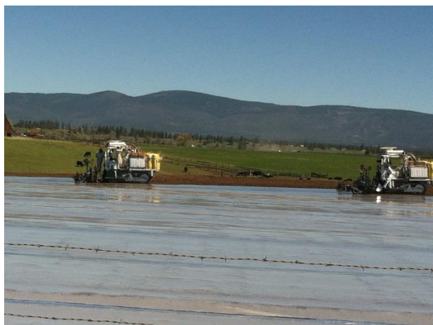
Pre-plant soil treatments involve specialized equipment which injects the pesticide directly into the soil. The area is immediately tarped and sealed for specified period of time to ensure maximum effectiveness of the treatment.
