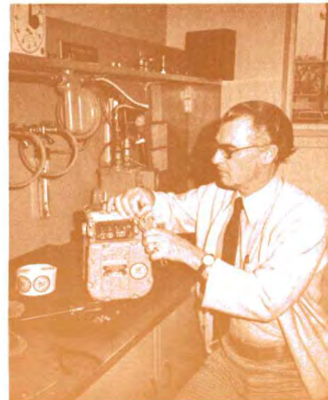
C. Bruce Wade - Sealer of Weights & Measures attaching seal to vapor meter.
