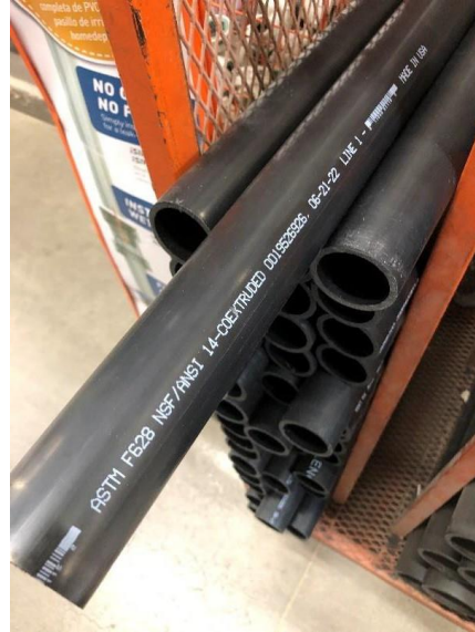
Non-potable/wastewater black PVC pipe
