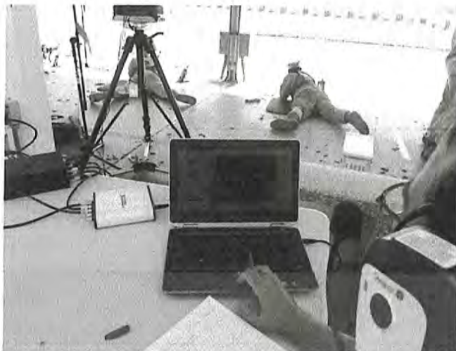
Figure 4: The NIOSH impulse noise measurement system being used at a military firing range. Microphones are positioned on
