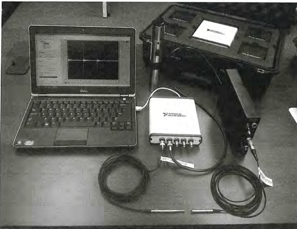
Figure 2: NIOSH Impulse Noise Measurement System Kit – consisting of a laptop running NIOSH Impulse Software, a National-Instruments (NI-4432) USB data acquisition board, and high-intensity microphones.
