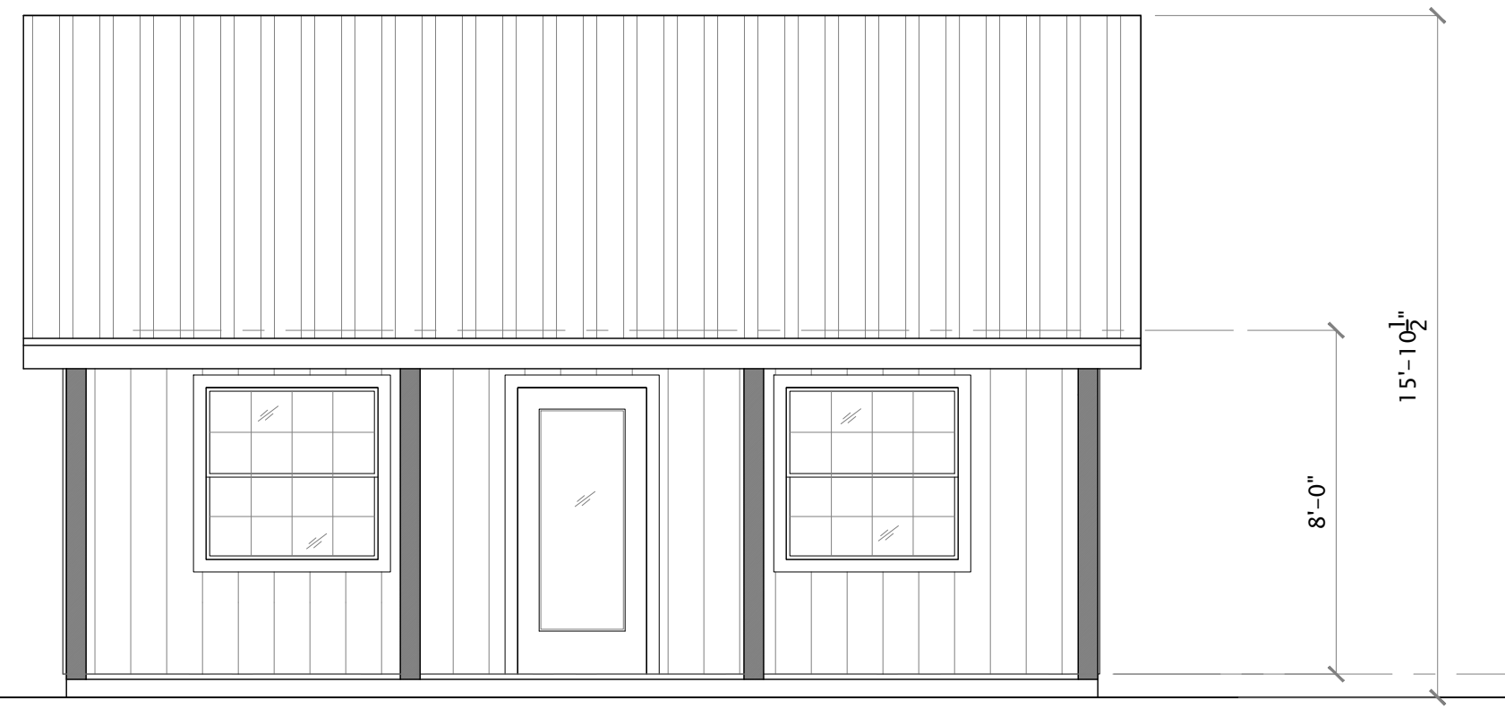
1 FRONT ELEVATION - OPTION A (GABLE ROOF) SCALE: 1/4" = 1'-0"
