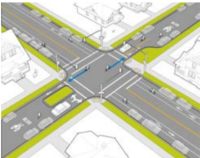
Figure 3.29. Example of a Class III Bicycle Boulevard with Traffic Diversion
